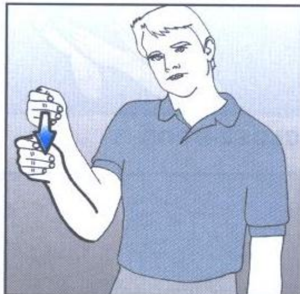
TURN-OFF (lever-type switch)
