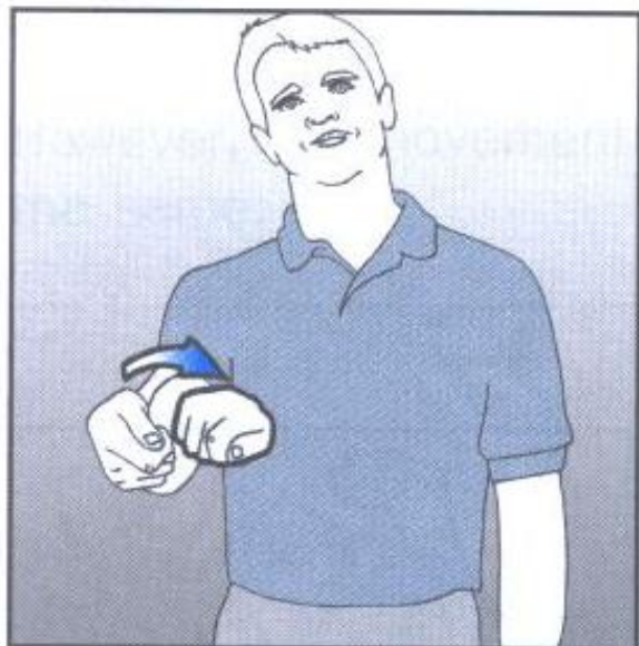
TURN-OFF (knob-type switch)
